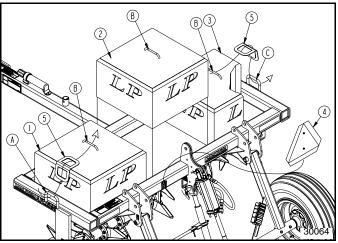
Concrete Weight Assembly (AR2596 Shown) Figure 2-2
